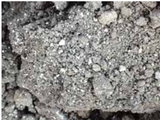
Figure 8. IXP ER ® 70C Calcium Peroxide blended into treatment pile soil
