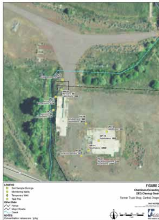
Figure 2. Soil boring locations of compounds found in exceedance of Oregon DEQ cleanup criteria
