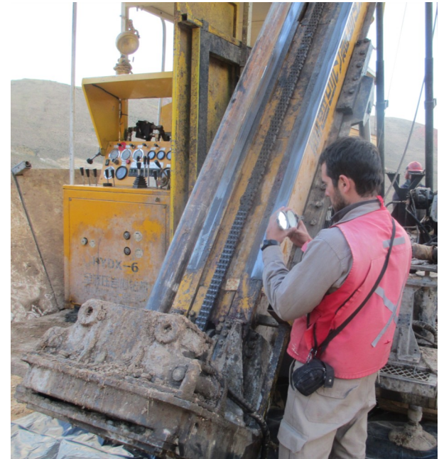
Geologist at drill rig checking the drill orientation at Chinchillas Deposit
