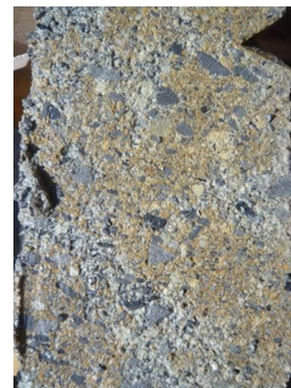
Typical Silver Mantos and Socavon del Diablo style fine grained disseminated sulphide
