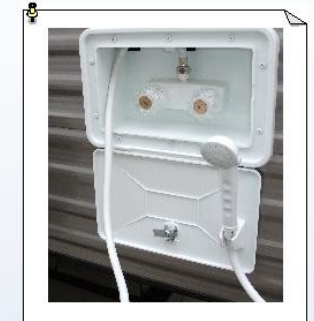
Standard outside shower offers hot and cold water access for washing off sand or filling the dog's water.
