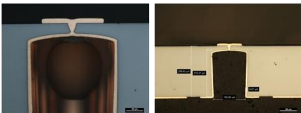
Figure 7. Cross-section of the finished metalized TSVs. The left shows a non-vacuum molded cross-section where a void is obtained while the right picture shows a vacuum molded cross-section.
