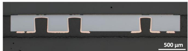
Figure 13. Cross section of a part of the 5 \times 3.5 \text{mm}^2 TSV interposer die embedded in mold compound without any air entrapments present in any hollow TSV after compression molding step but before \mu -via drilling and fan-out process steps.
