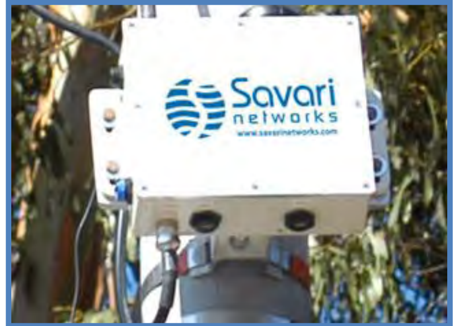
Pole Mounted Roadside Equipment (RSE)
