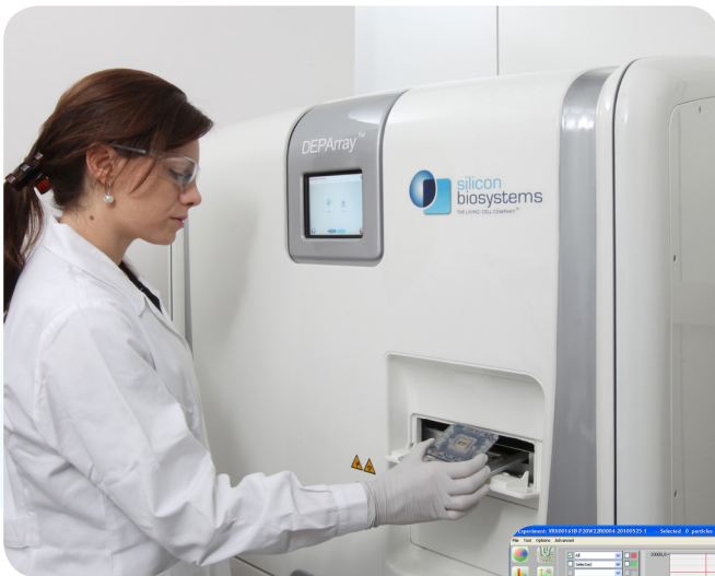
The DEPArray™ instrument for imaged-based cell selection and collection.
