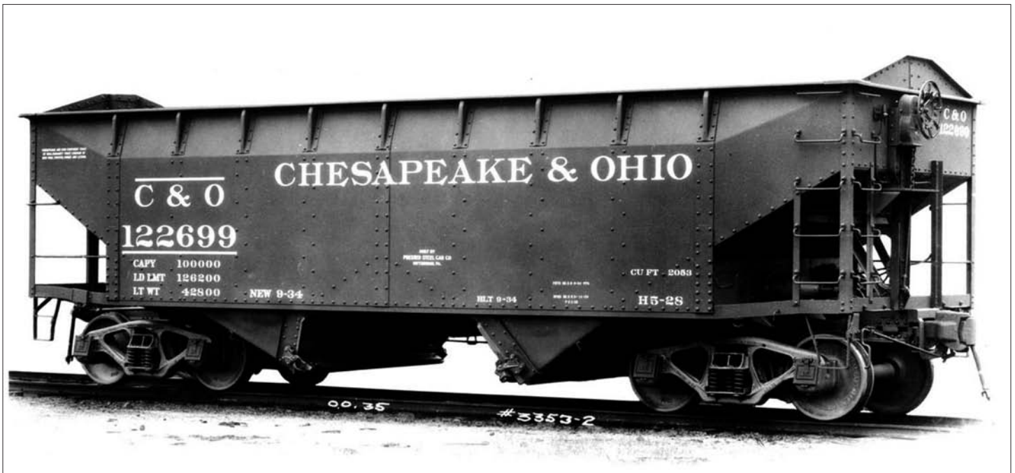
This builder's photo of C&O No. 122699 clearly shows the angular end extension that was standard on most of the cars in this group. Also clearly visible is the geared handbrake mechanism, characterized by the vertical brake wheel.
