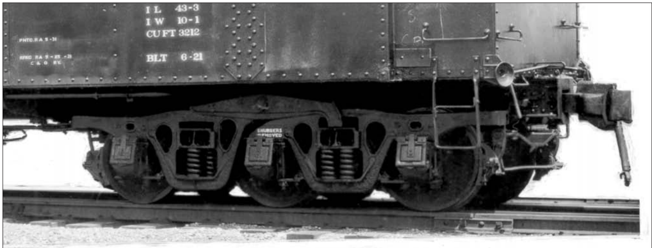
Replacement 100-ton American Steel Foundries "equalized" six-wheel trucks with 50-ton journals and axles and clasp brake shoes, installed at Clifton Forge and Newport News in 1924 under the 91-ton 100000-series gondola cars. The cars were then placed in test service for an extensive shakedown period. These trucks stayed under these cars until they were retired in 1946.
