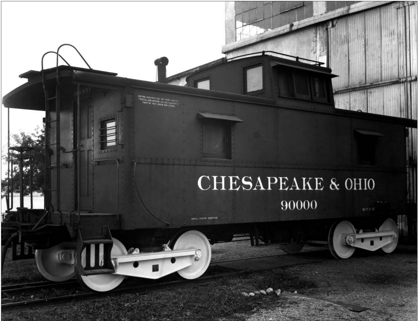
Steel caboose No. 90000, the first of its type on the C&O, was experimentally fitted with Difco axleless trucks. The experiment was apparently not considered to be a success, since these are the only photographs we have of this interesting installation.
