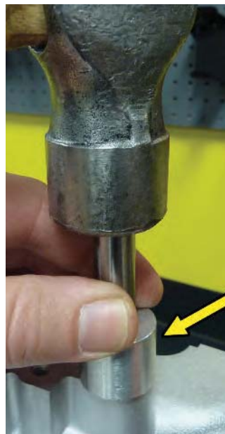
Driving plug into galley bore. Note how the squaring sleeve keeps driver perpendicular to the head.
