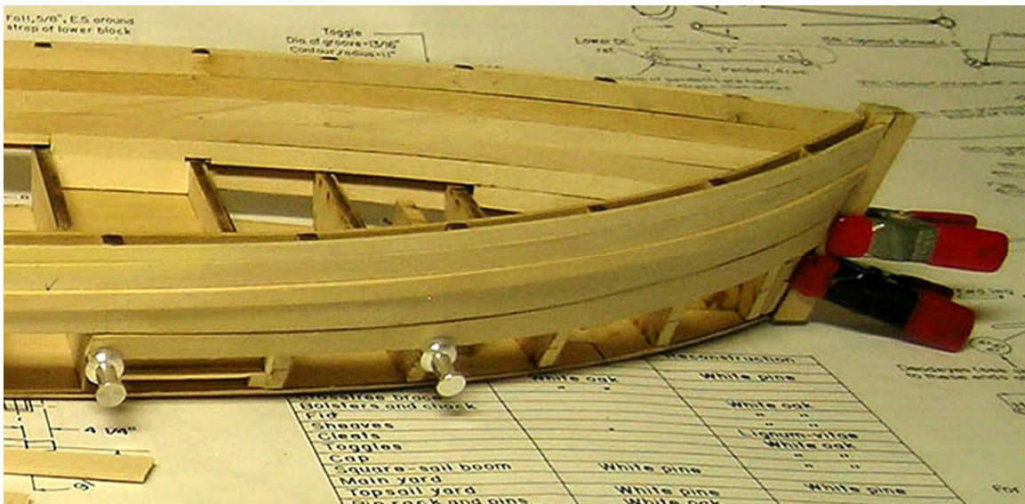
Photo 3: method of clamping planks
