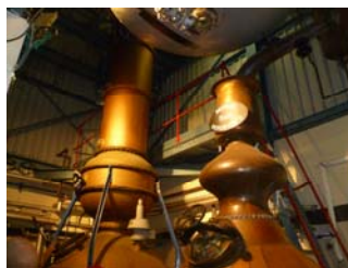
Above: Hendrick's Carter-Head still, which bathes the botanicals in vapor, was originally built in 1948 and is one of only a handful remaining in the world. The copper pot Bennett Still, which boils the botanicals, is one of the oldest in the industry, dating to 1860.
